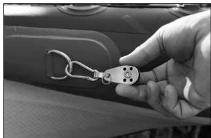
Fig 23: Attach the pulleys
